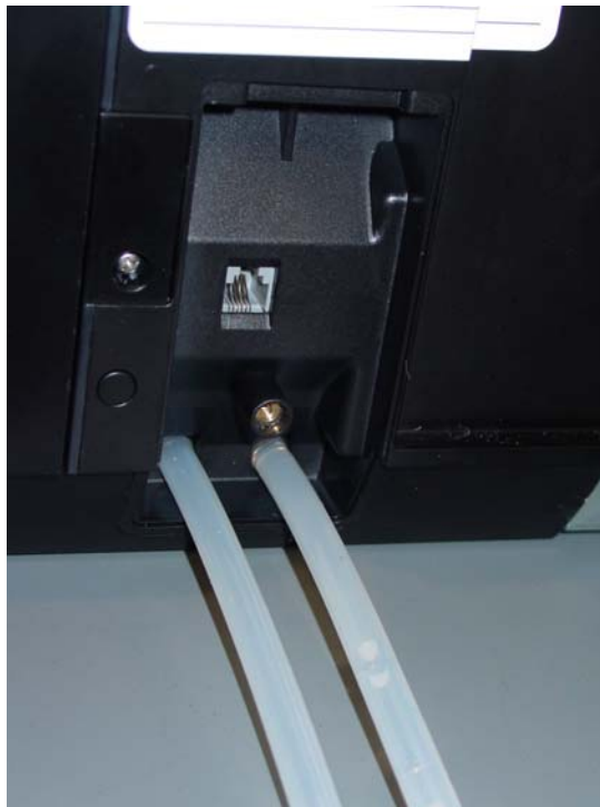
Drain Tubes with Access Panel removed
