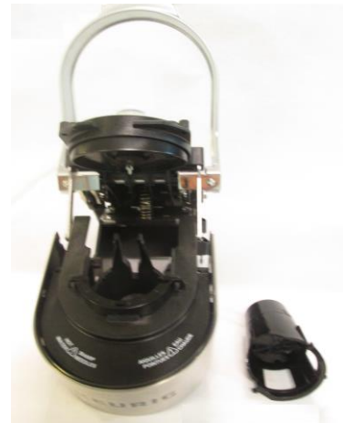
9. THE POD HOLDER, LOWER RIGHT, SHOULD BE REMOVED AND SANITIZED AS DESCRIBED IN THE USE & CARE GUIDE.
