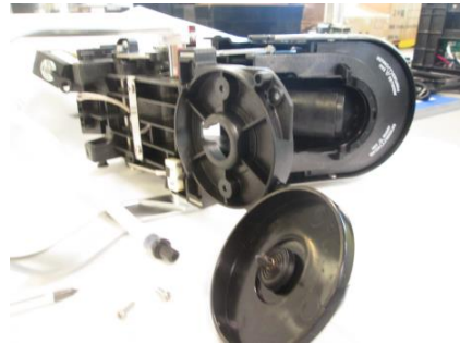
6. HERE THE PM IS SHOWN WITH THE PM ENTRANCE NEEDLE REMOVED.
