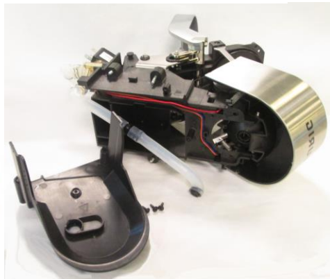
5. REMOVE UPPER PM ENTRANCE NEEDLE COVER BY REMOVING THE TWO SCREWS AS INDICATED
