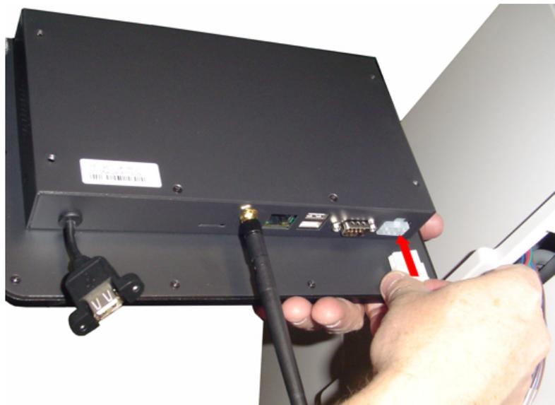
7. Place the HMI onto the door, making certain to secure the USB connector to its retainer on the door.
