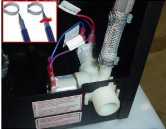
2. Disconnect the wiring from the inlet valve. **Be careful not to discard or misplace the small blue jumper wire.**
