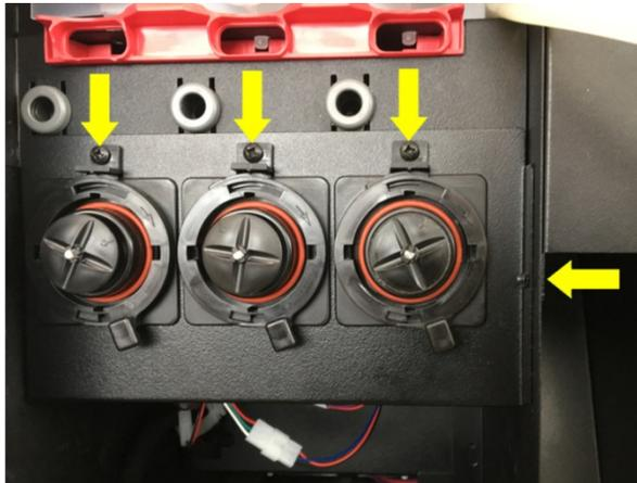
3. Disconnect the inline power connector to the blower.
