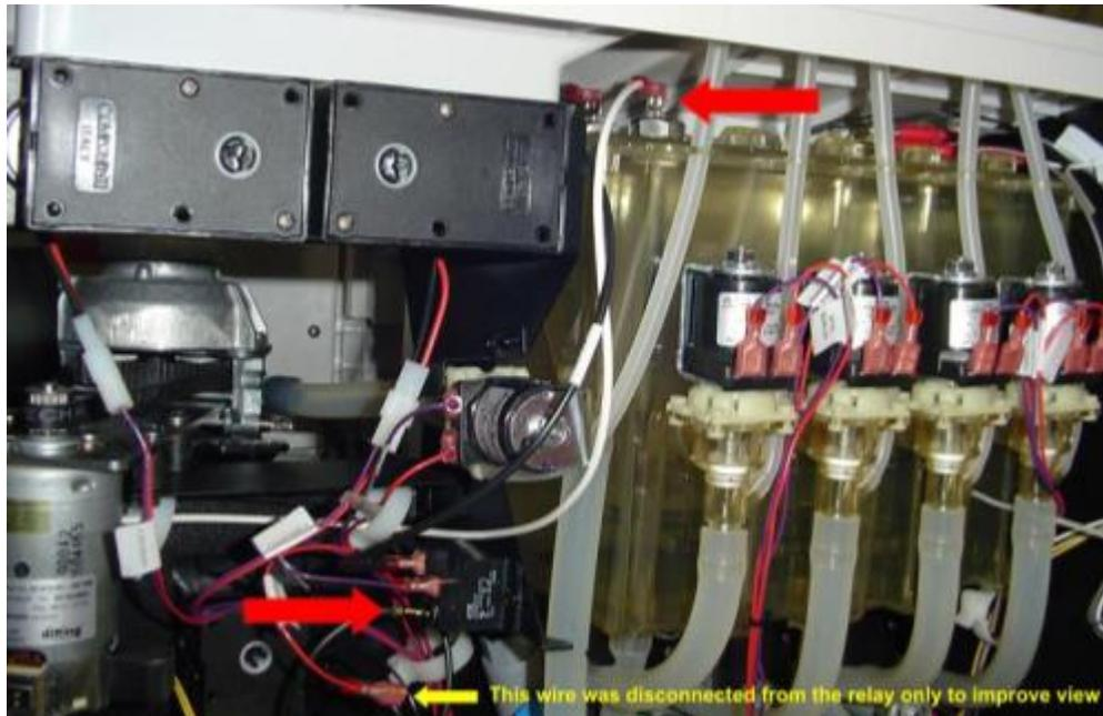
9. Reconnect the black wiring pair to the fuse holder.
