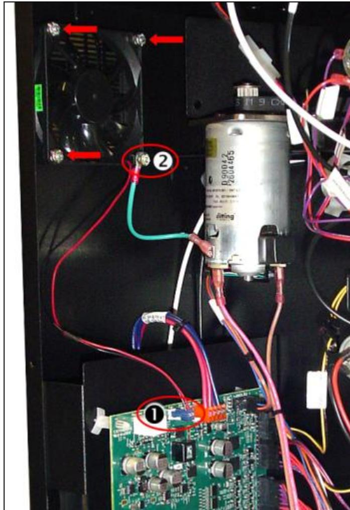
1. With the back panel removed, disconnect the exhaust fan wiring from the control board.
