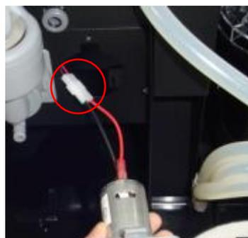
2. Install the new motor into the cutout in the machine wall. Install the bottom of the assembly first, and then push the top of the assembly into the cutout until the plastic clip locks it in place.
