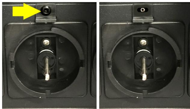
7. Push down on the locking clip at the front of the base, and pull the base and motor out through the front of the support.
