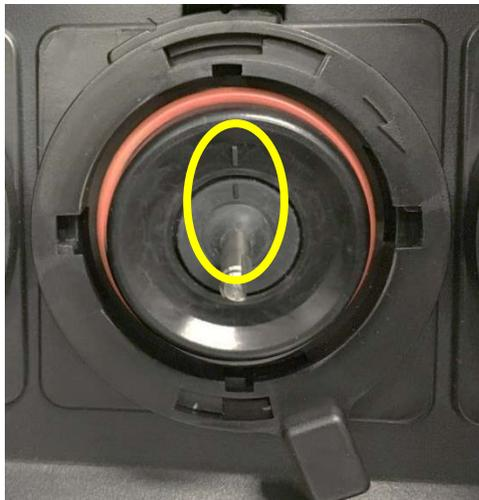
When replacing the **impeller**, align the small arrow on the impeller with the flat side of the whipper shaft. Push the impeller until it clicks in place.
