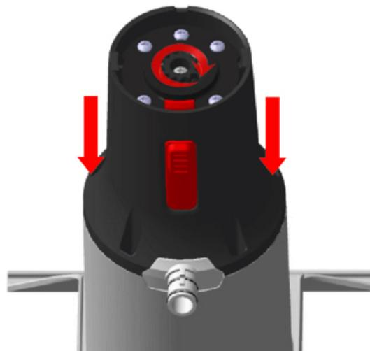
10. Insert the five screws into the cylinder base and tighten them in the sequence shown.
