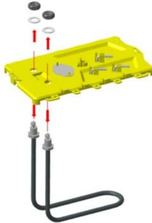
2. Insert the new heating element through the bottom of the tank lid, and secure it to the top using the large hex nuts and washers.
