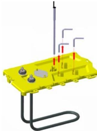
2. Slide the new temperature probe and/or water level probes completely into the tank lid until they are clipped and locked in position.
