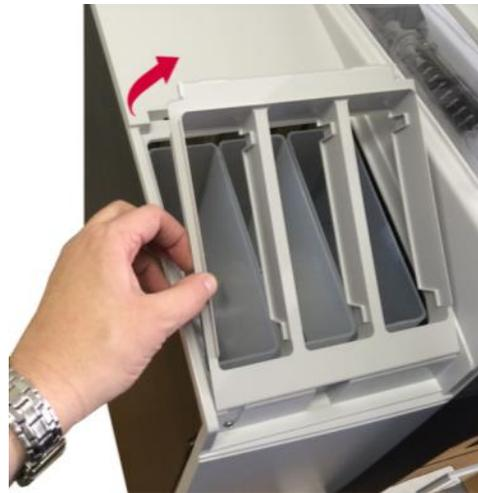
4. Lift the top front of the dispenser, while at the same time pulling the bottom of the dispenser forwards to disengage the coupling from the dispenser motor.
