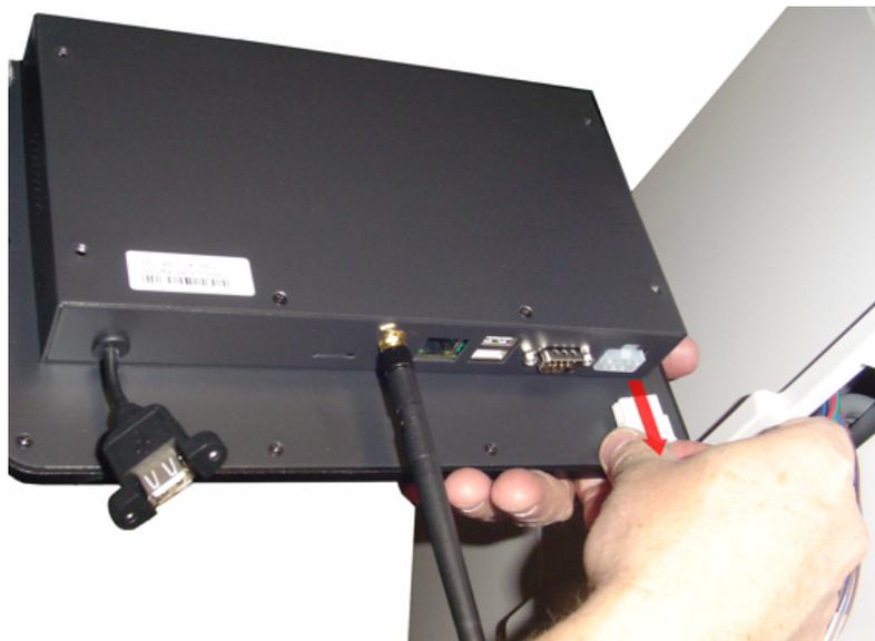
5. Install the antenna onto the bottom of the HMI (if missing).
