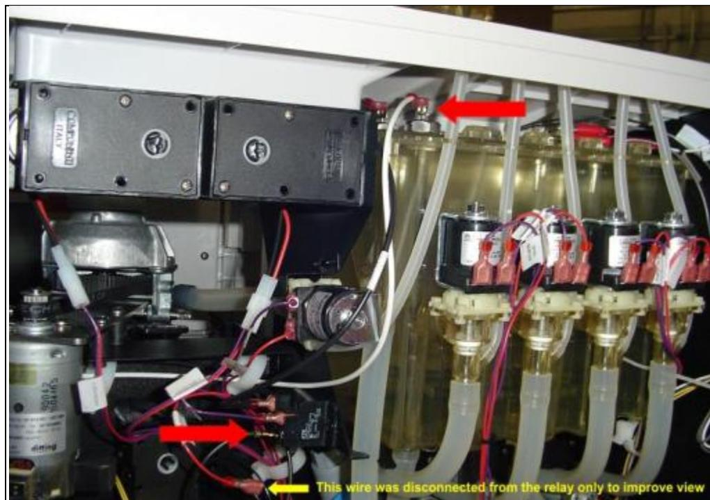
6. Remove the black and white wires (going to the heating circuit) from the wire clips.
