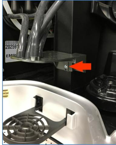
3. Remove the residue chute by pulling the top section outwards while lifting the chute.
