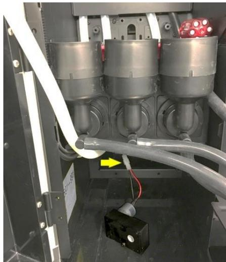
4. Disconnect the inline wiring connector for the motor to be removed (yellow arrow).
