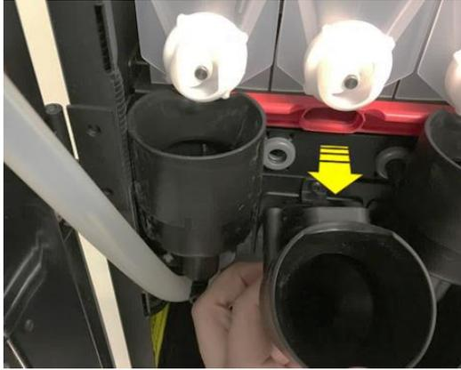
4. Remove the impeller from the motor shaft.
