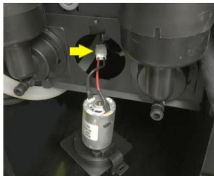
2. Install the new motor into the cutout in the machine wall. Install the bottom of the assembly first, and then push the top of the assembly into the cutout until the plastic clip locks it in place.
