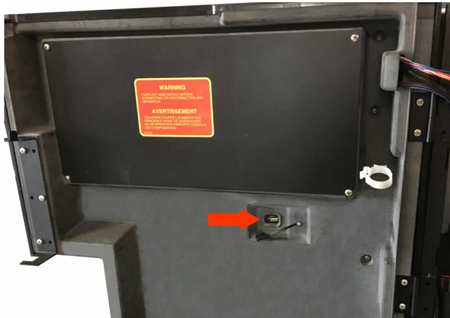
4. Reboot the machine using the main power switch (switch the power off for 5 seconds and then on again).
