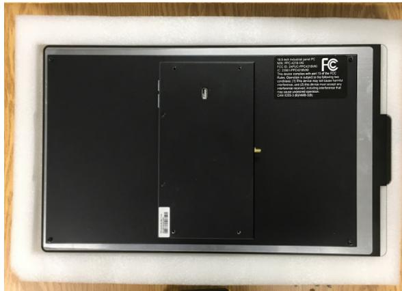
7. Remove the old HMI from the foam support and place the new HMI onto the support.
