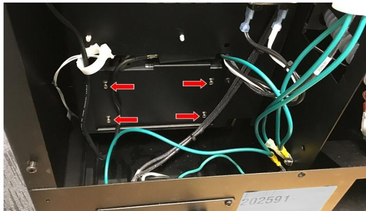
7. From the front of the machine, lift and pull out the power supply.
