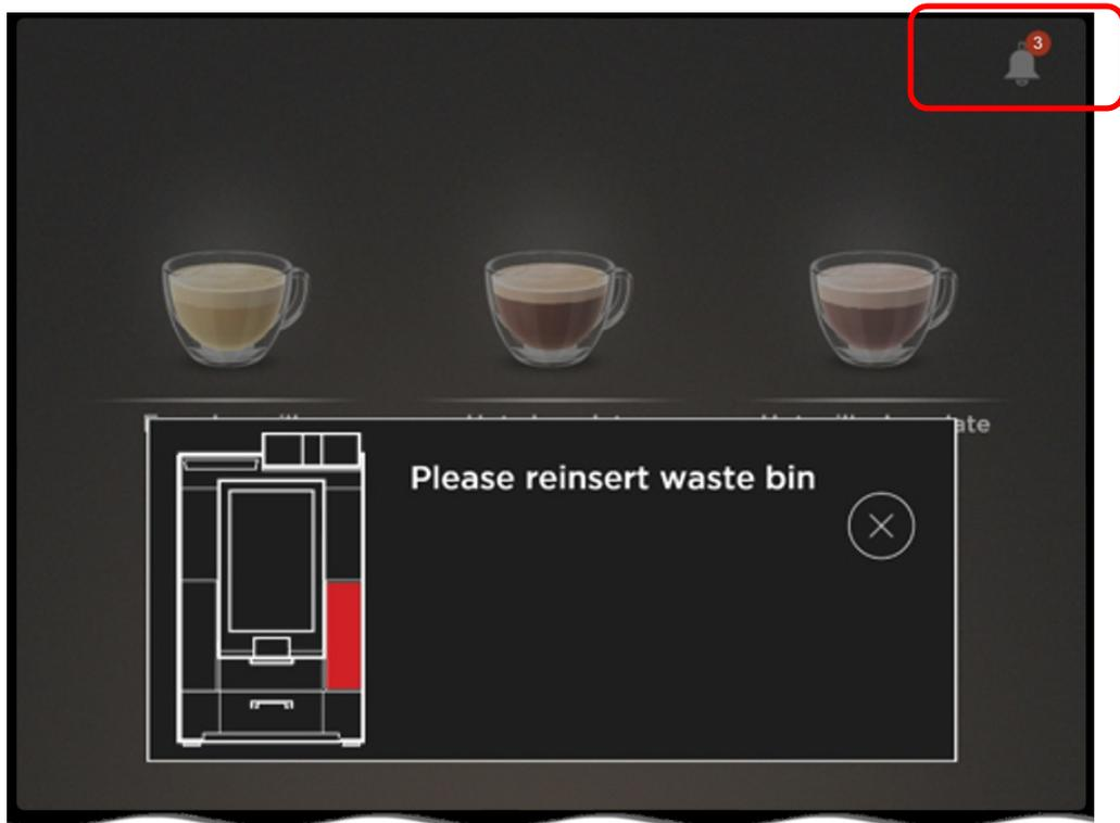
In this case, the waste bin has been removed and its presence is not detected. The waste bin must be replaced to clear this message.
