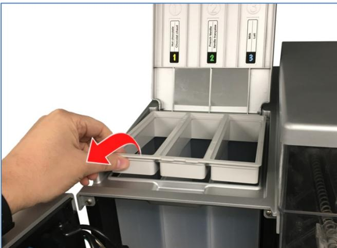
3. Lift the front of the dispenser and pull it forwards and out of the machine.
