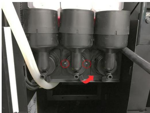
3. Remove the whipper chamber and the steam trap from the whipper base, disengaging it from the powder drawer and inlet fitting.
