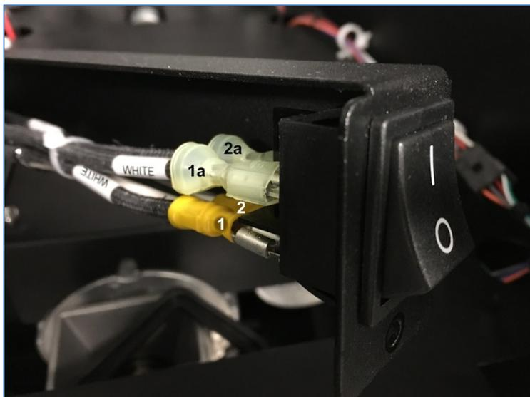
7. Re-install the secondary switch plate and secure it in place with two screws.
