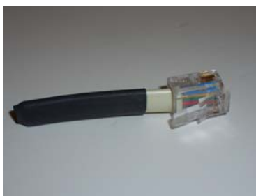
Figure 1. Modified RJ11 cable for coin unit test
