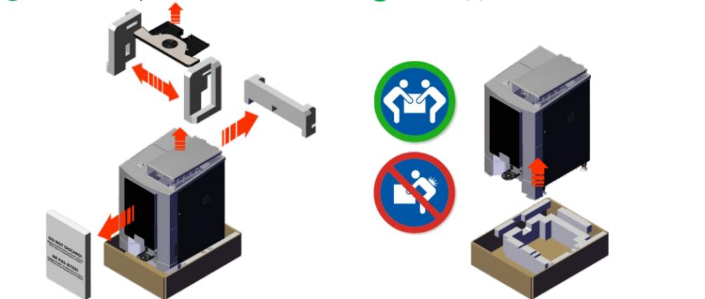
**3** Remove the four foam supports and remove the cup stand secured between the two upper supports. **Do not discard the front support as it must be installed over the machine's screen to protect it when transporting the machine.**
